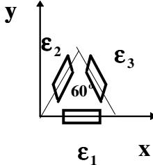
$$\begin{aligned}\varepsilon_1 &= \varepsilon_x \cos^2 0^\circ + \gamma_{xy} \sin 0^\circ \cos 0^\circ \\ &\quad + \varepsilon_y \sin^2 0^\circ\end{aligned}$$
