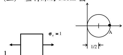
$$\begin{aligned}\sigma_{max} &= 1 & \theta_p &= 0 \\ \sigma_{min} &= 0 & \theta_p &= \pi/2 \\ \tau_{max} &= 1/2 & \theta_s &= \pm\pi/4 \\ \sigma_s &= 1/2\end{aligned}$$
