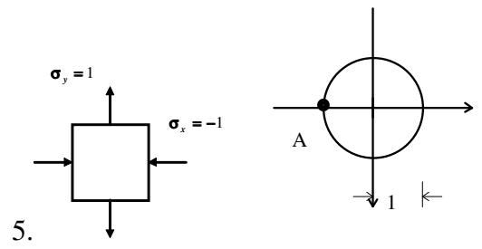
$$\begin{aligned}\sigma_{max} &= 1 & \theta_p &= \pi/2 \\ \sigma_{min} &= -1 & \theta_p &= 0 \\ \tau_{max} &= 1 & \theta_s &= \pm\pi/4 \\ \sigma_s &= 0\end{aligned}$$
