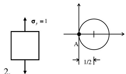
$$\begin{aligned}\sigma_{max} &= 1 & \theta_p &= \pi/2 \\ \sigma_{min} &= 0 & \theta_p &= 0 \\ \tau_{max} &= 1/2 & \theta_s &= \pm\pi/4 \\ \sigma_s &= 1/2\end{aligned}$$
