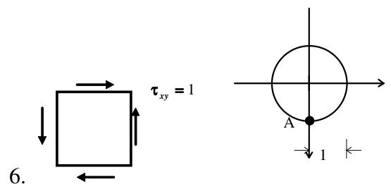
$$\begin{aligned}\sigma_{max} &= 1 & \theta_p &= \pi/4 \\ \sigma_{min} &= -1 & \theta_p &= -\pi/4 \\ \tau_{max} &= 1 & \theta_s &= 0, \pi \\ \sigma_s &= 0\end{aligned}$$
