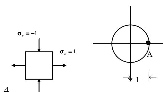
$$\begin{aligned}\sigma_{max} &= 1 & \theta_p &= 0 \\ \sigma_{min} &= -1 & \theta_p &= \pi/2 \\ \tau_{max} &= 1 & \theta_s &= \pm\pi/4 \\ \sigma_s &= 0\end{aligned}$$
